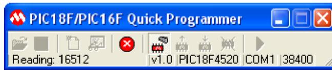
Once the read has been completed, “Finished operation...” will be displayed. This verifies that board is correctly connected to the PC and the communication settings are correct.
