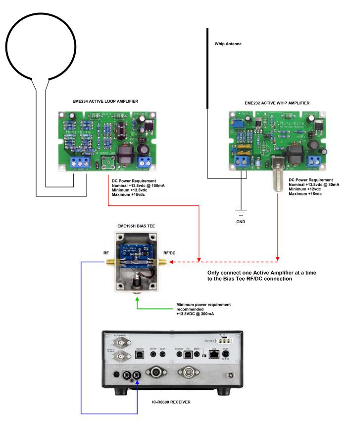
After installation, DC Power should be measured on the Active Amplifier after the Voltage Regulator to make sure that it is close to +12vdc for best operation of the amplifier.
