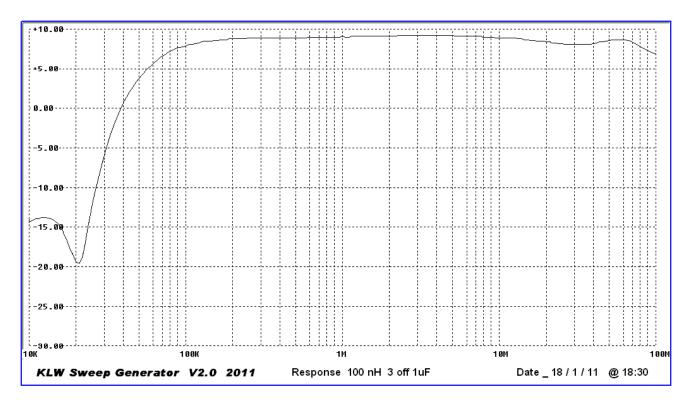
With 100 nH replacing 10 nH and 3 off 0.1 uF increased to 1.0 uF
