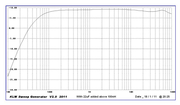
Inductor supply bypassed with 22 uF electro plus 100 uH plus 1.0 uf feed capacitors
